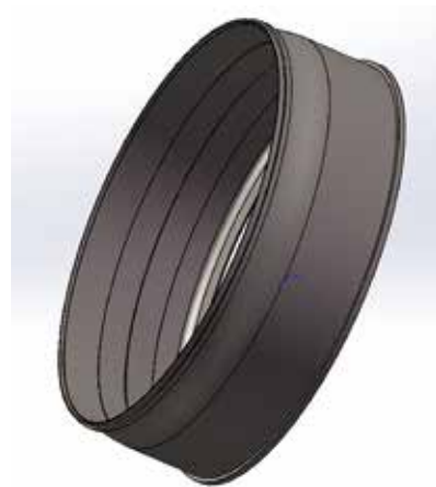
图2 薄壁机匣三维模型 Fig.2 Three-dimensional model of thin-walled casing
