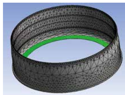
图3 薄壁机匣有限元网格划分后的模型和约束(绿色部分0位移约束) Fig.3 Thin-walled casing finite element meshing model and constraint (green part is 0 displacement constraint)
